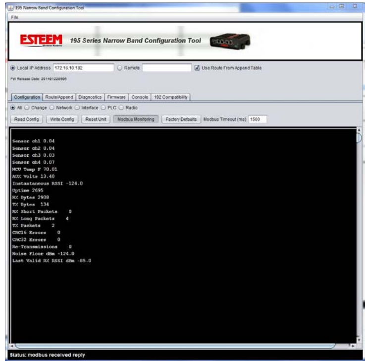
Figure 7: Modbus Monitoring Screen
