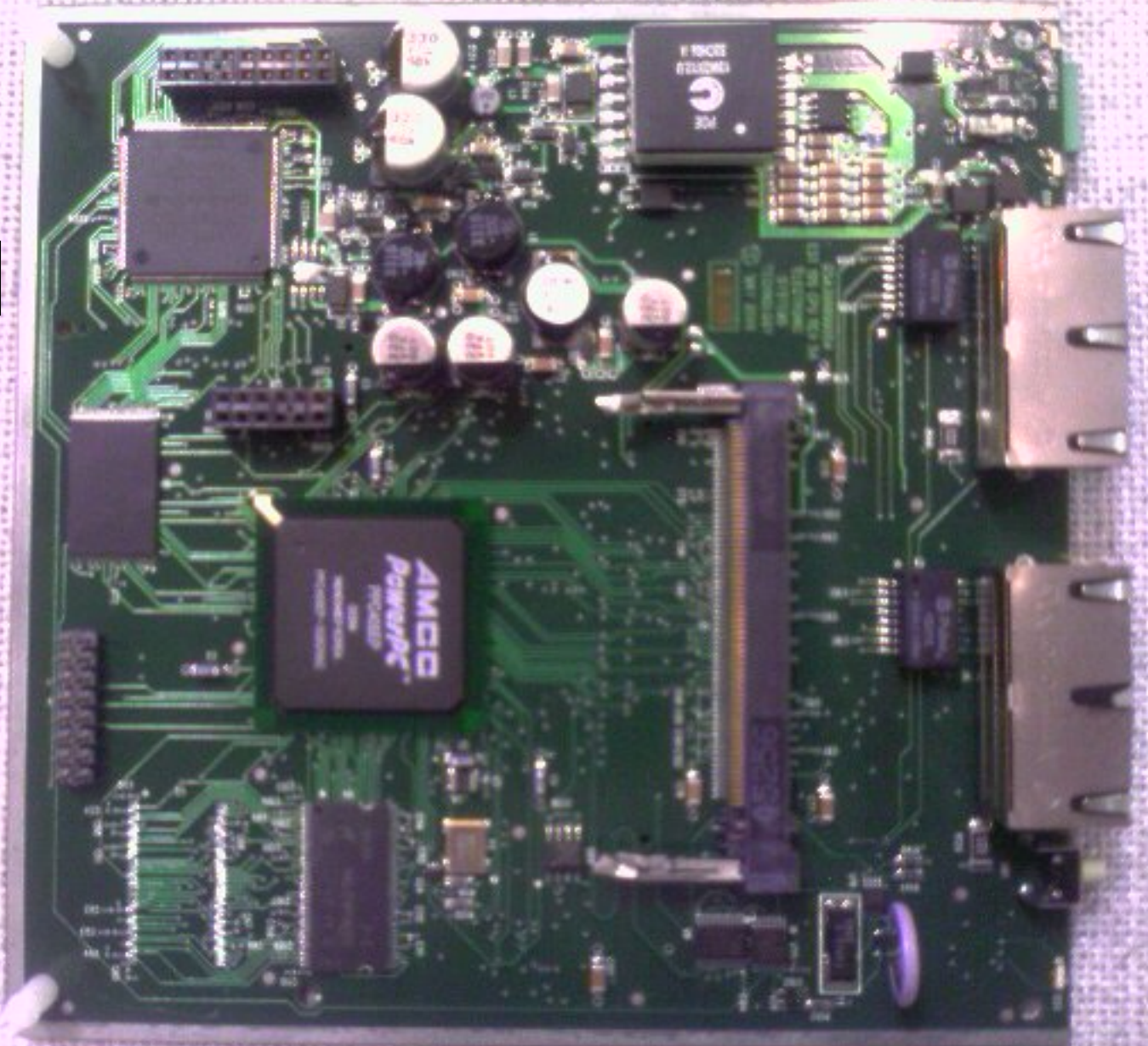
Main Board Top with Radio Card Removed
