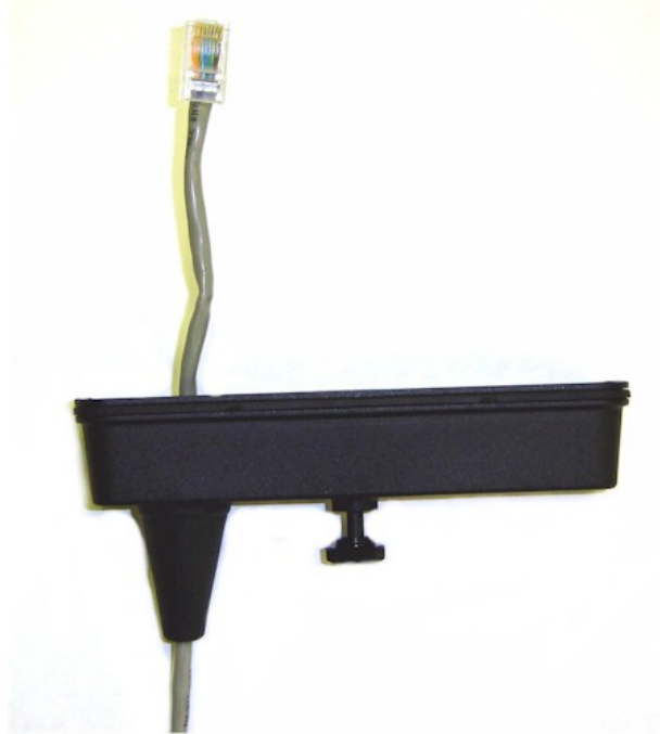
Figure 7: Ethernet Cable Routing
