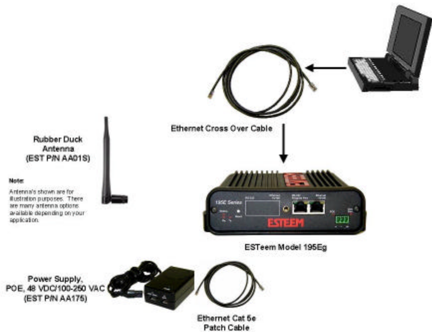
Figure 2: Hardware Setup Direct to Computer
