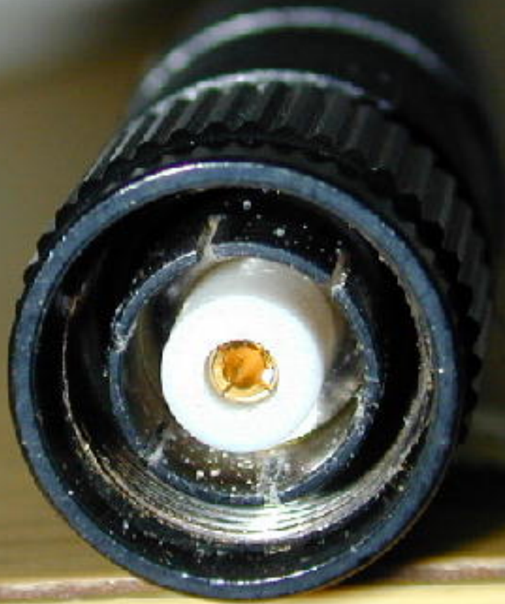
"Ducky" Antenna Connector - Reverse TNC
