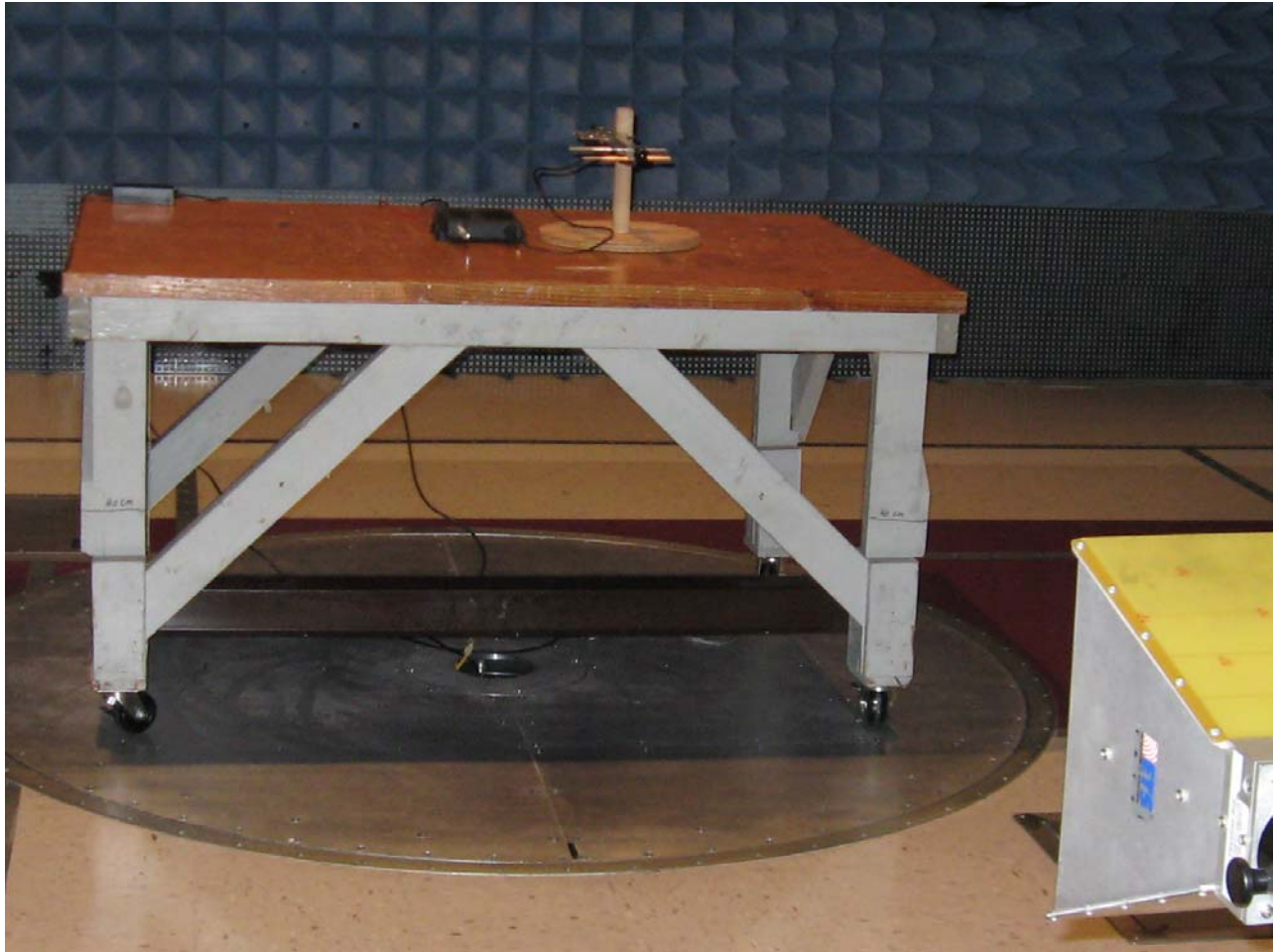
Photograph 8. Test Equipment and setup for various Radiated Measurements (Yagi Antenna)
