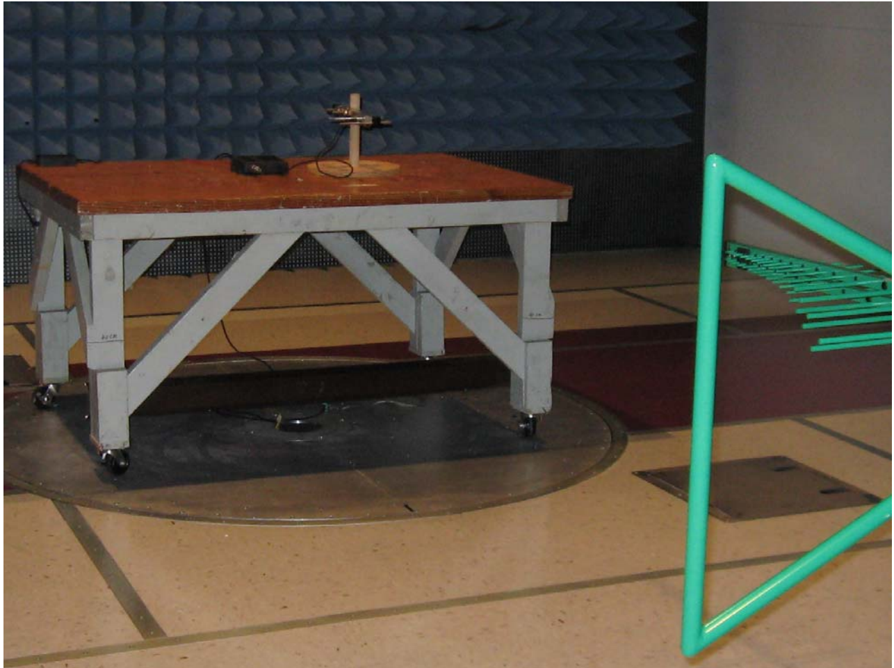
Photograph 4. Radiated Emission Test Setup 30 MHz - 1 GHz, Yagi Antenna
