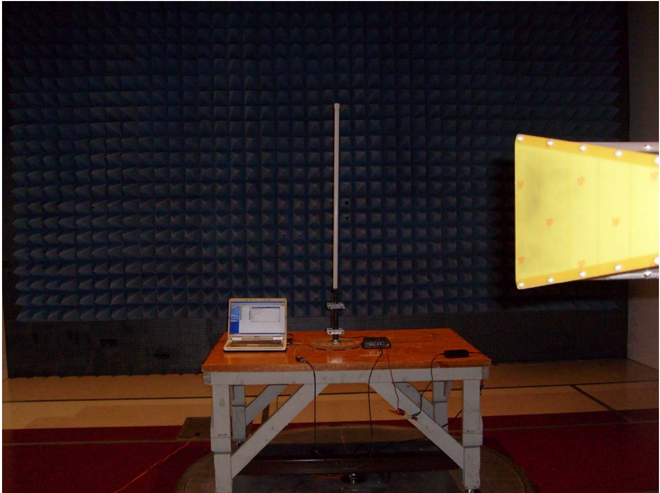
Photograph 9. Test Equipment and setup for various Radiated Measurements (Omni Antenna)
