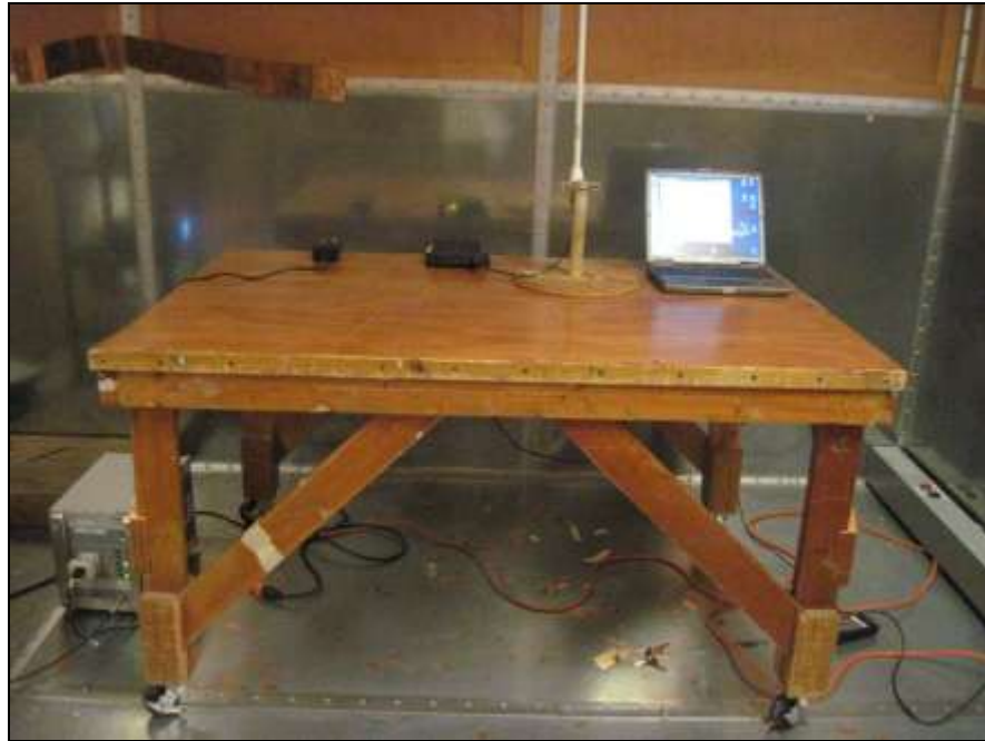
Photograph 10. Conducted Emissions, 15.207(a), Test Setup, POE (1)
