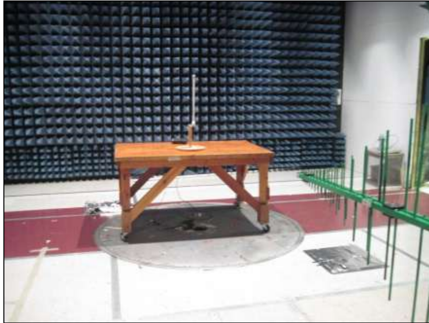
Photograph 12. Radiated Spurious Emissions, Test Setup, Omni Antenna, 30 MHz – 1 GHz
