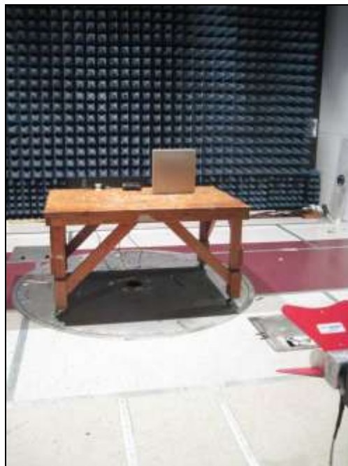
Photograph 7. Radiated Emissions, Test Setup, Above 1 GHz
