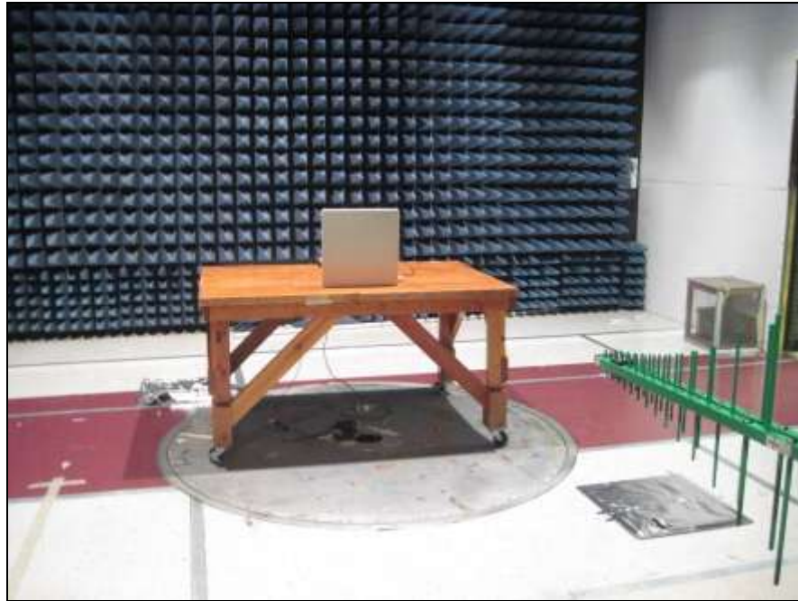
Photograph 14. Radiated Spurious Emissions, Test Setup, Panel Antenna, 30 MHz – 1 GHz
