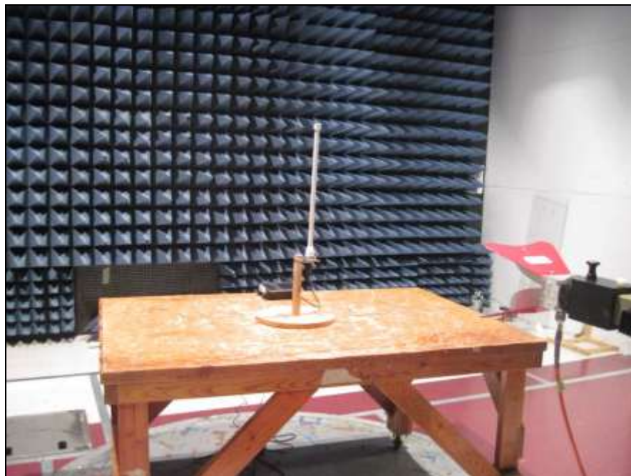
Photograph 13. Radiated Spurious Emissions, Test Setup, Omni Antenna, Above 1 GHz
