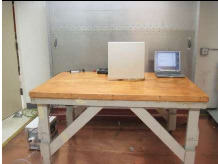
Photograph 8. Conducted Emissions, 15.207(a), Test Setup, AC/DC (1)
