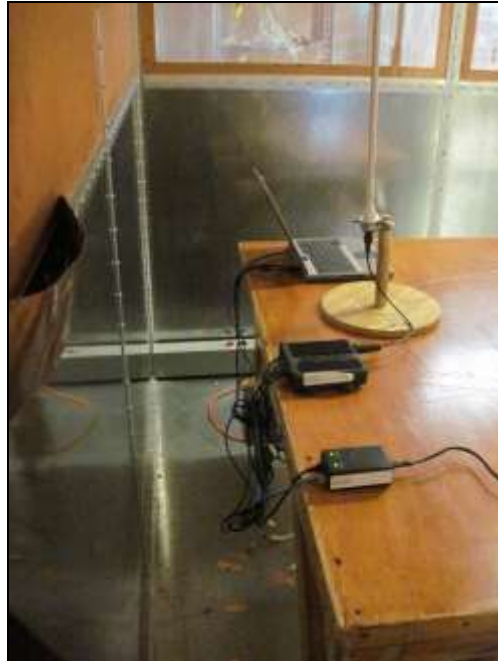
Photograph 11. Conducted Emissions, 15.207(a), Test Setup, POE (2)
