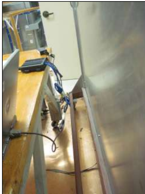
Photograph 9. Conducted Emissions, 15.207(a), Test Setup, AC/DC (2)
