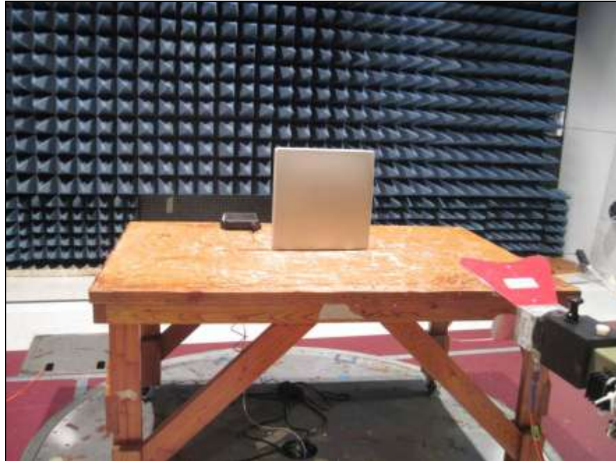
Photograph 15. Radiated Spurious Emissions, Test Setup, Panel Antenna, Above 1 GHz
