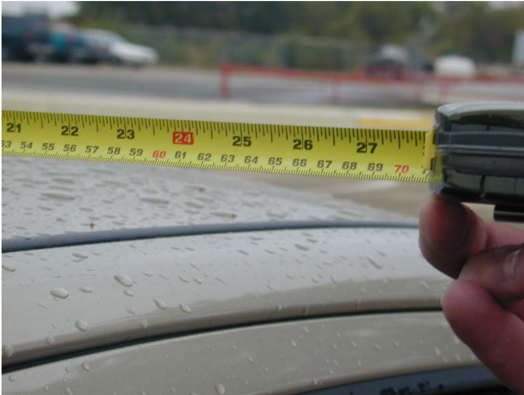
Distance from center of antenna to edge of roof – 60 cm.
