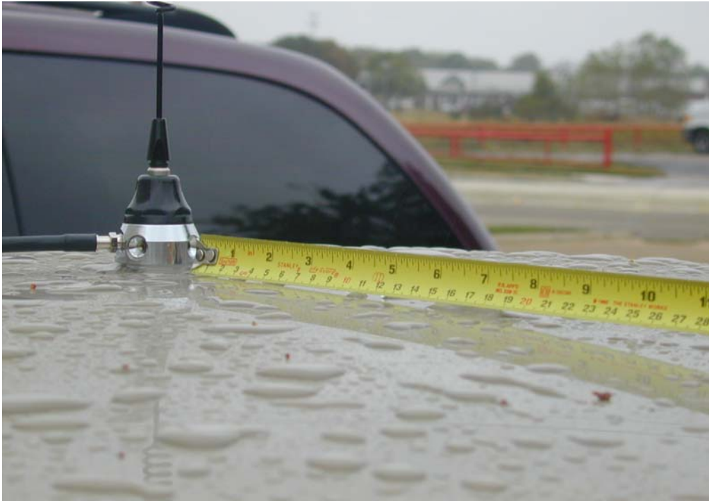
Antenna in center of roof
