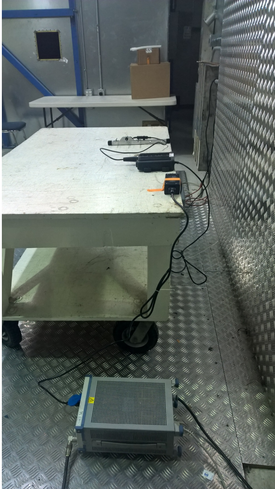
Figure 8.2-3: Conducted disturbance at mains port setup photo
