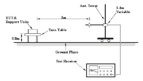
The radiated emission tests were performed in the 3-meter chamber test site, using the setup accordance with the ANSI C63.10-2013. The specification used was the FCC Part Subpart C limits.
