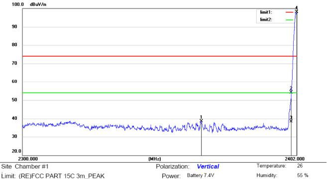
Limit: (RE)FCC PART 15C 3m\_PEAK Mode: DTS (TX2402)
