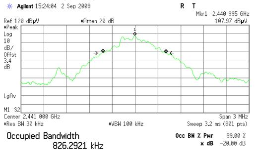
Transmit Freq Error -5.743 kHz x dB Bandwidth 845.826 kHz
