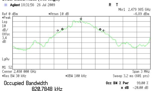
Transmit Freq Error -5.910 kHz x dB Bandwidth 857.556 kHz
