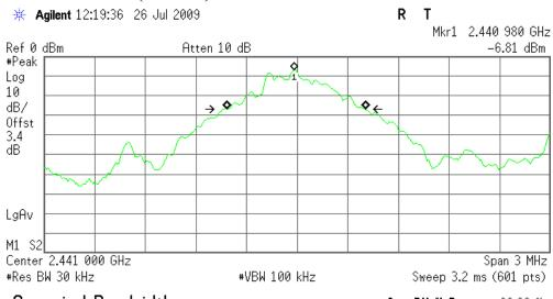
Occupied Bandwidth 821.5808 kHz Occ BW % Pwr 99.00 % x dB -20.00 dB
