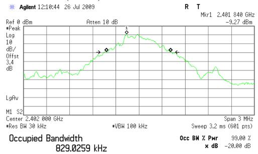
Transmit Freq Error -3.750 kHz x dB Bandwidth 872.293 kHz
