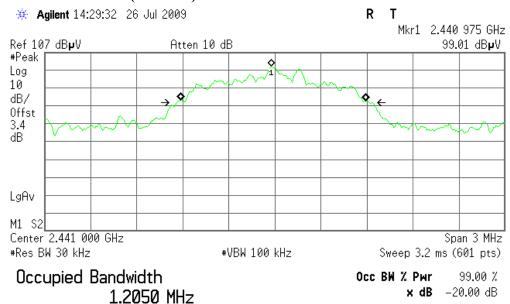
Transmit Freq Error -13.915 kHz x dB Bandwidth 1.257 MHz
