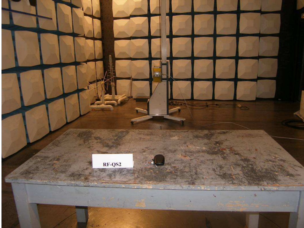
Photograph 6: Set-up for Spurious Emissions (18GHz-26GHz)
