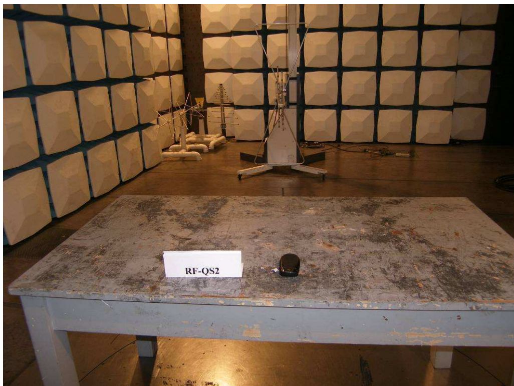
Photograph 4: Set-up for Spurious Emissions (30MHz-1GHz)
