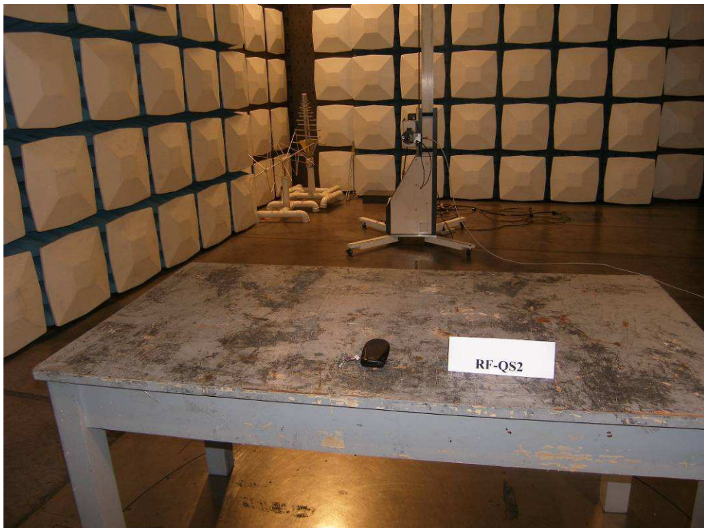
Photograph 6: Set-up for Spurious Emissions (18GHz-26GHz)
