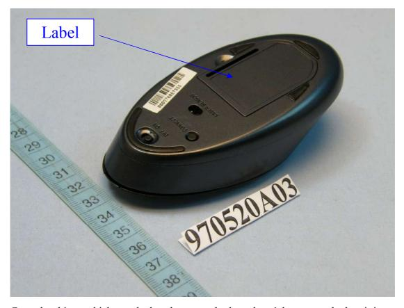
Cover has hinge which attached to the mouse body and can't be removed when it is at open position
