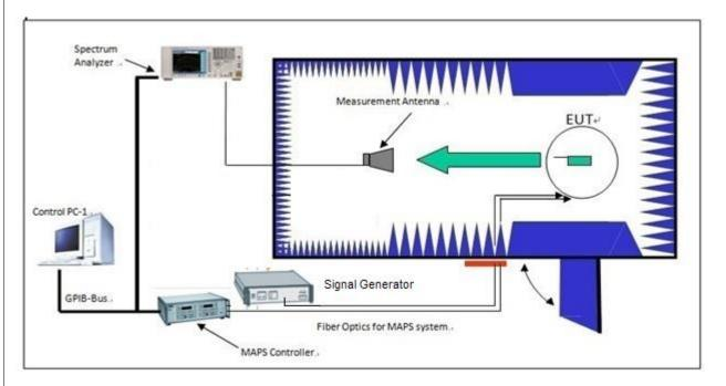
Figure 1. 2D antenna pattern test system.
