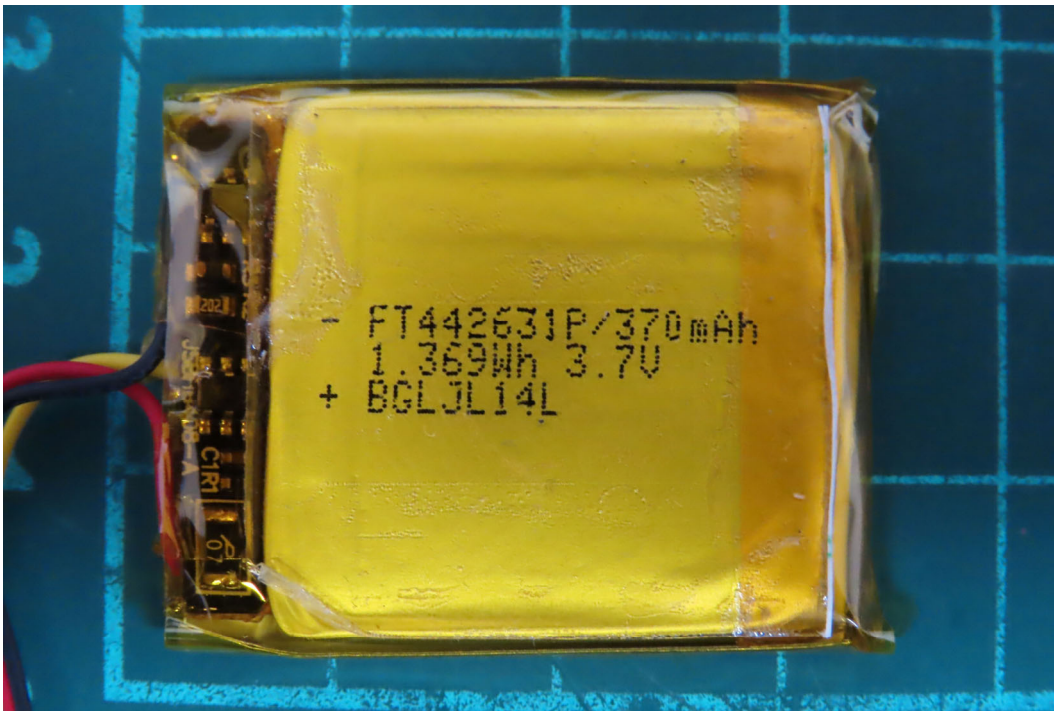
(6) EUT Photo - Battery - MFR: Hangzhou Future Power Technology Co., Ltd. Model No.: FT442631P/370mAh
