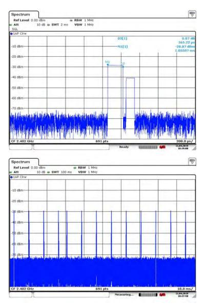
Time on of 100ms= 165.2us\*13= 2.147ms Duty Cycle=2.147ms / 100ms= 0.06 Duty Cycle correction factor= 20 LOG 0.06= -33.363 dB
