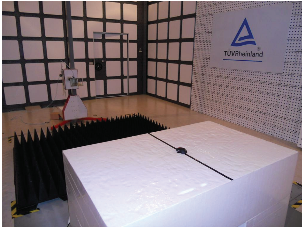
Photograph 3: Set-up for Spurious Emissions (Back View 2)
