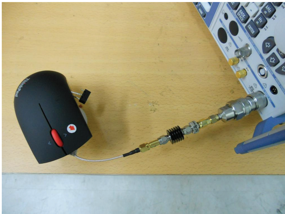
Photograph 4: Set-up for Conducted testing
