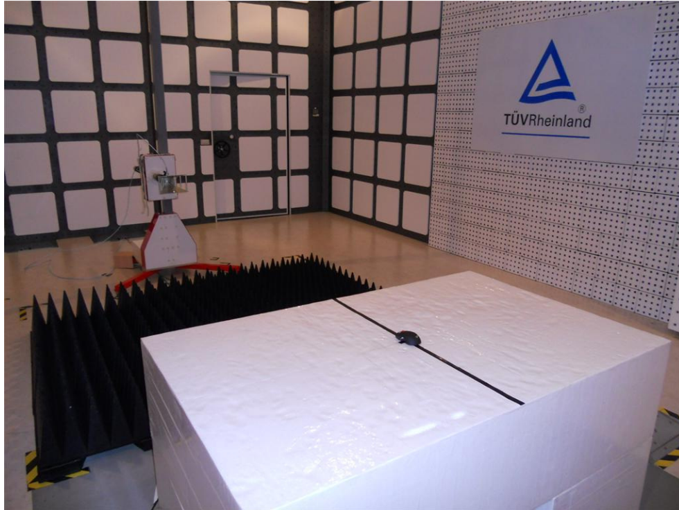
Photograph 3: Set-up for Spurious Emissions (Back View 2)
