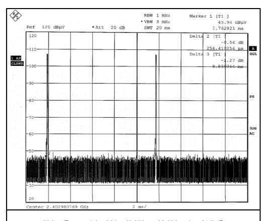
$20 \log (Duty cycle) = 20 \log (0.256 \text{ ms} / 9.839 \text{ ms}) = -31.7 \text{ dB}$
