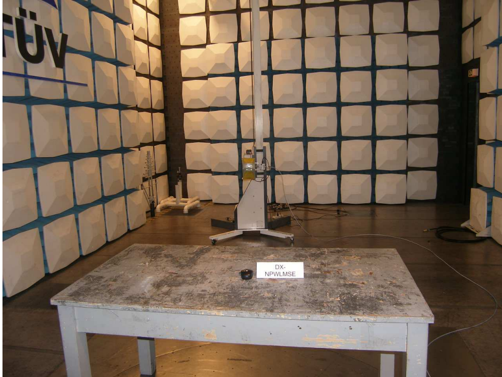
Photograph 4: Set-up for Radiated Emissions (18GHz-25GHz)
