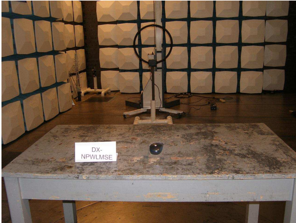
Photograph 2: Set-up for Radiated Emissions (30MHz-1GHz)
