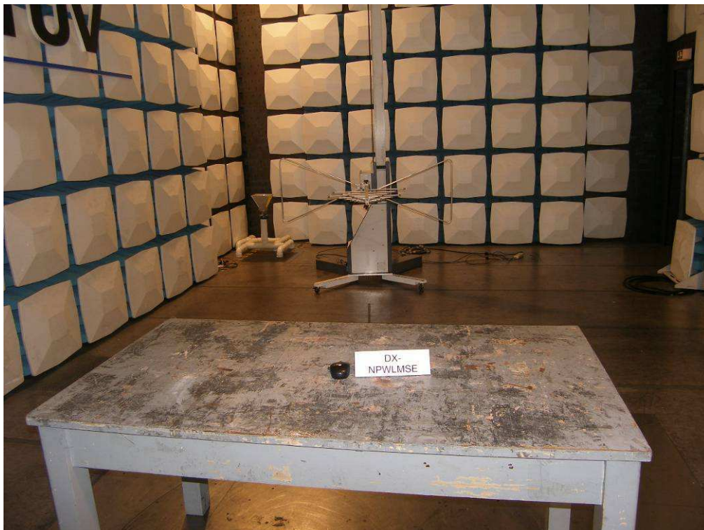
Photograph 2: Set-up for Radiated Emissions (30MHz-1GHz)
