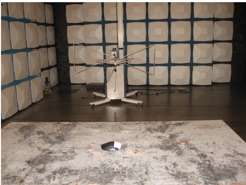
Photograph 2: Set-up for Emissions (30MHz-1GHz)
