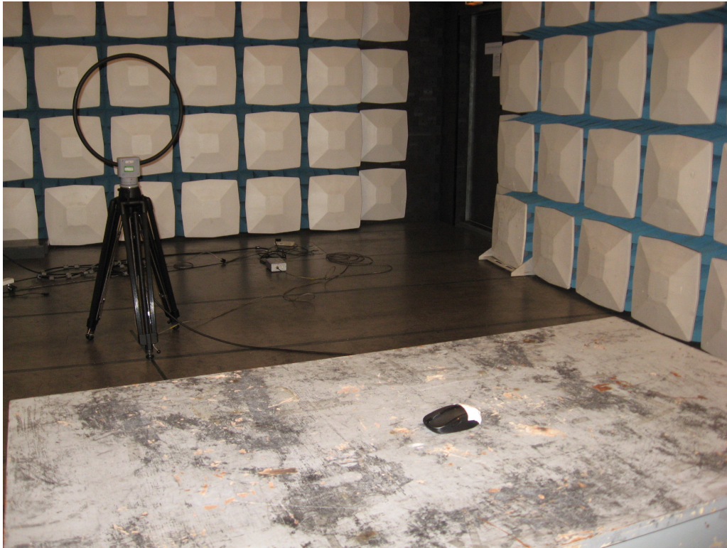
Photograph 2: Set-up for Emissions (30MHz-1GHz)
