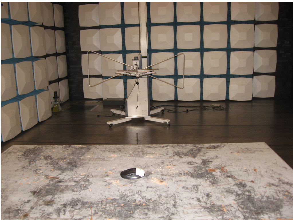
Photograph 2: Set-up for Emissions (30MHz-1GHz)
