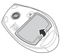
2 Pull the receiver out of the battery compartment.
