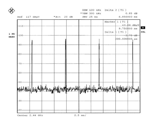
$$20\log(\text{Duty cycle}) = 20\log\frac{0.2 \text{ ms}}{6.85 \text{ ms}} = -30.69 \text{dB}$$
