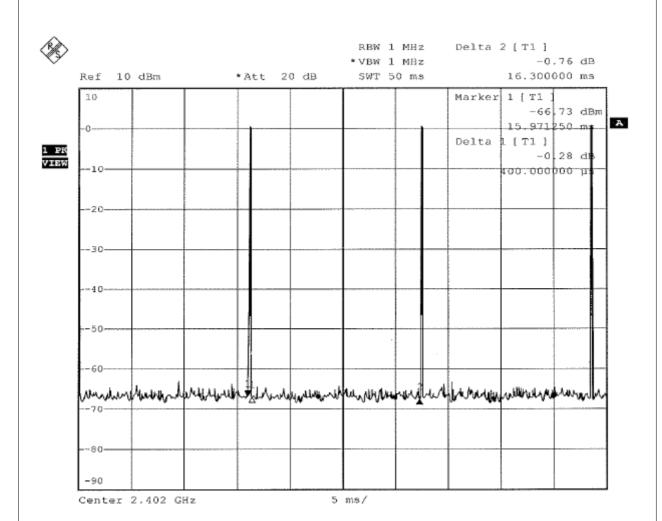
$$20\log(\text{Duty cycle}) = 20\log\frac{0.4 \text{ ms}}{16.3 \text{ ms}} = -32.2 \text{dB}$$
