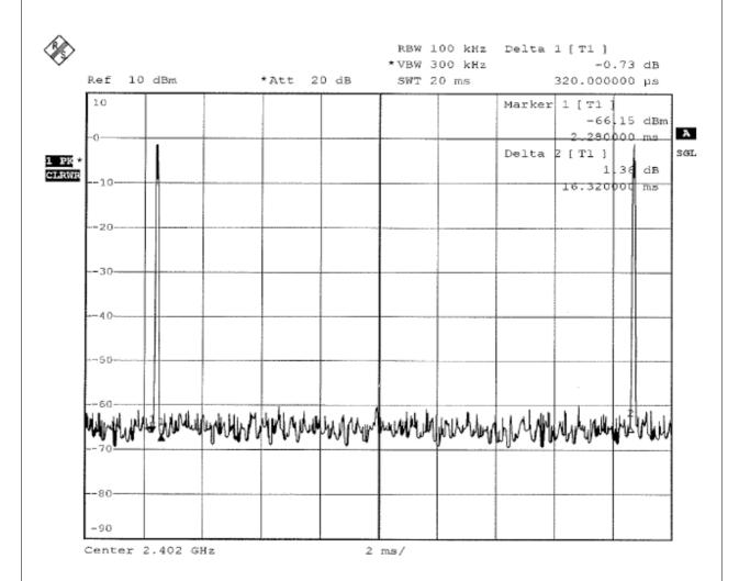
$$20\log(\text{Duty cycle}) = 20\log\frac{0.32 \text{ ms}}{16.32 \text{ ms}} = -34.15 \text{dB}$$
