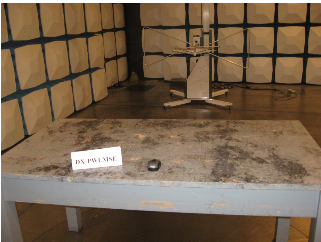
Photograph 2: Set-up for Emissions (30MHz-1GHz)
