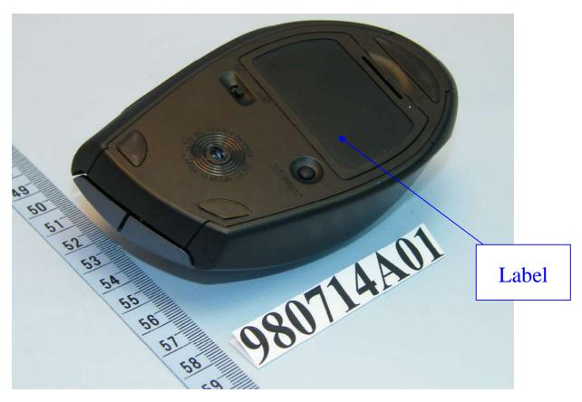
Cover has hinge which attached to the mouse body and can't be removed when it is at open position
