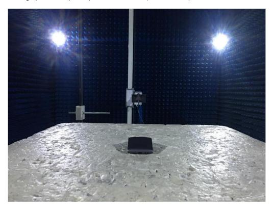
Photograph 4: Set-up for Spurious Emissions (18GHz-26GHz)
