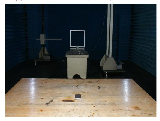
Photograph 2: Set-up for Spurious Emissions (30MHz-1GHz)
