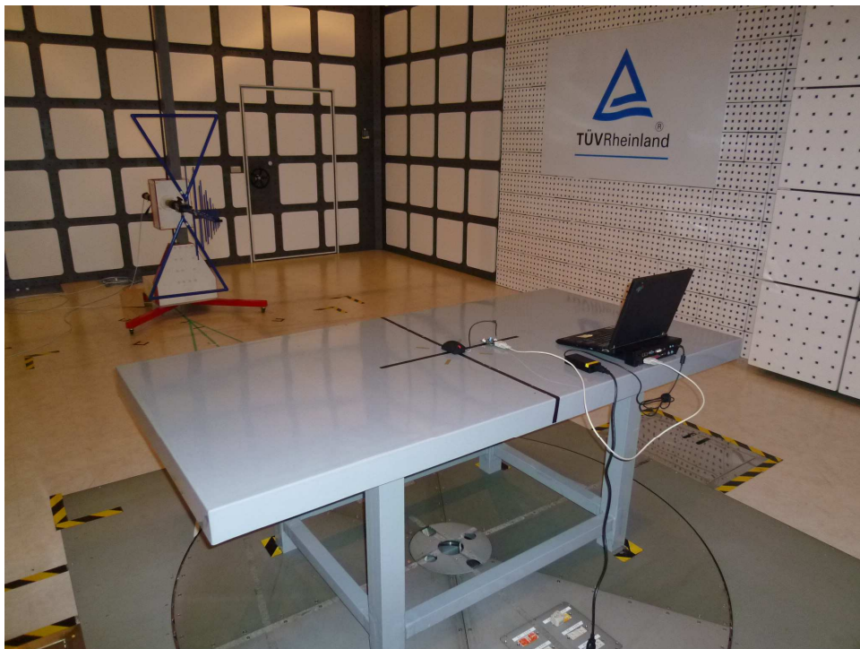
Photograph 2: Set-up for Spurious Emissions (Back View 1)
