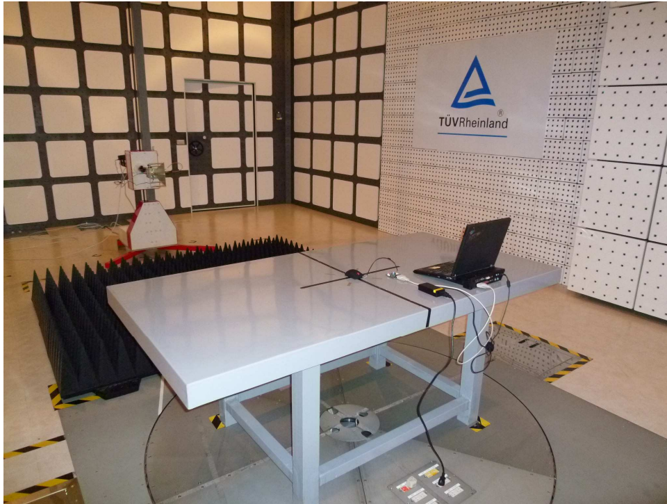
Photograph 4: Set-up for Conducted testing
