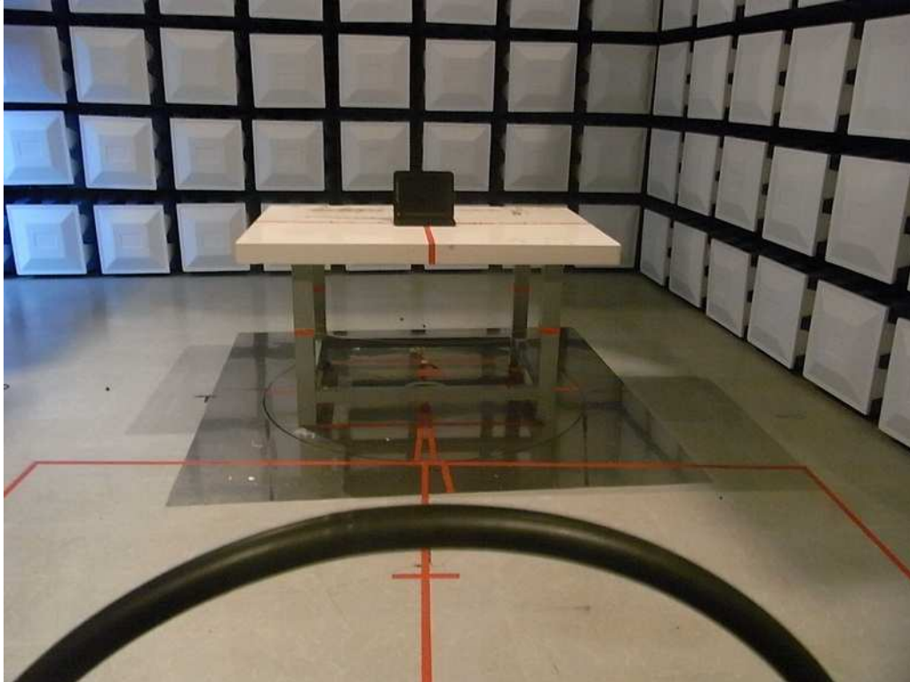
Photograph 2: Set-up for Spurious Emissions (30MHz-1GHz)
