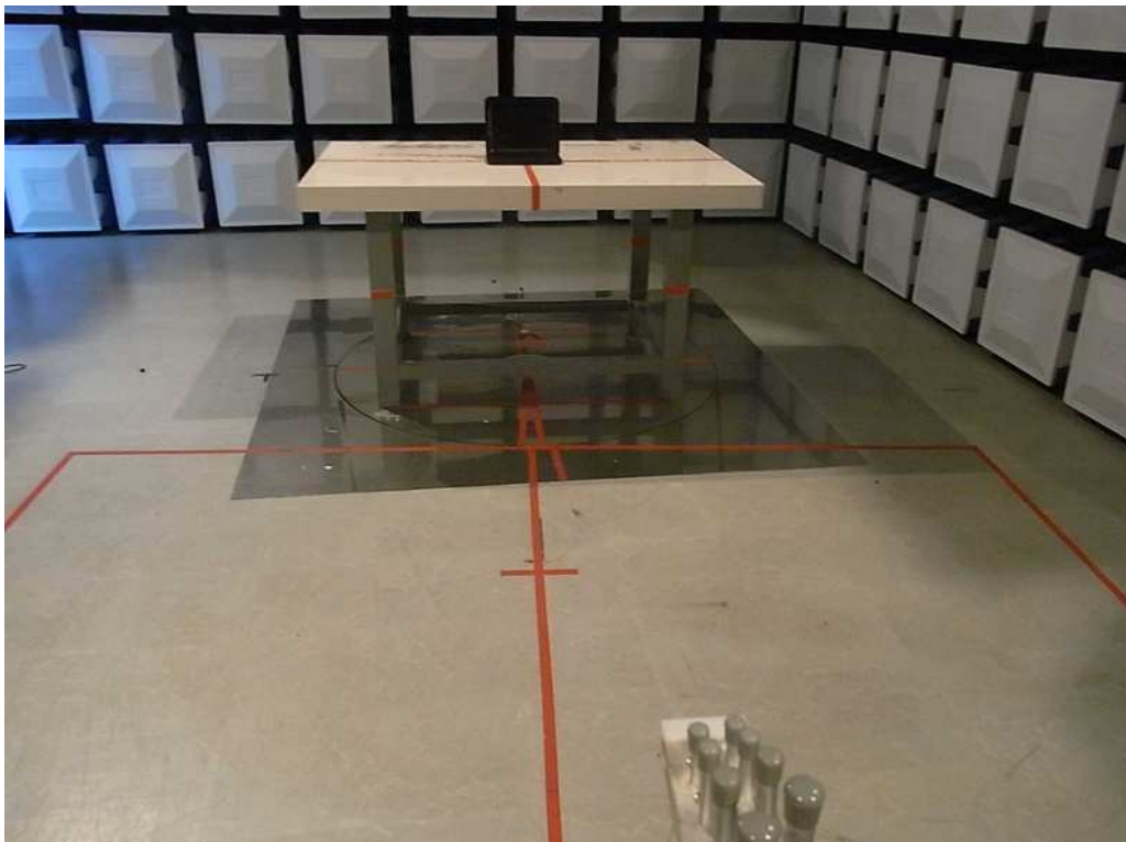
Photograph 2: Set-up for Spurious Emissions (30MHz-1GHz)
