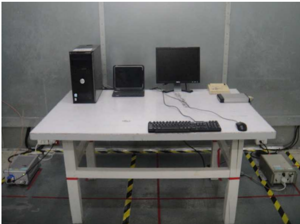
Photograph 6: Set-up for Conducted emissions
