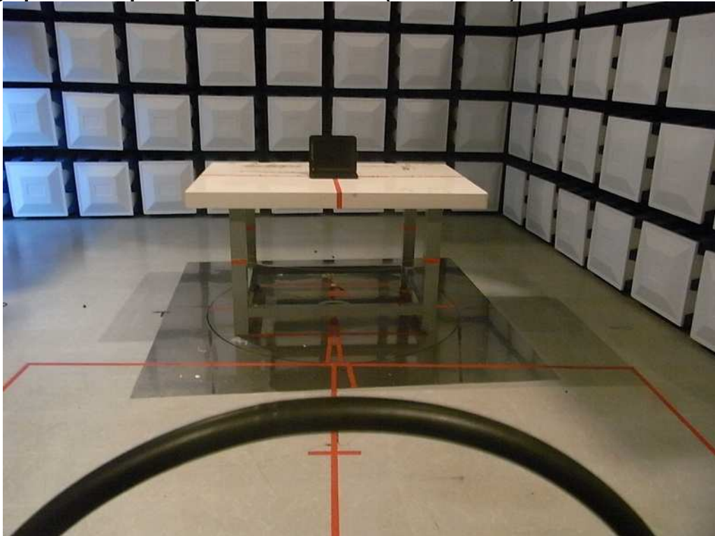
Photograph 2: Set-up for Spurious Emissions (30MHz-1GHz)
