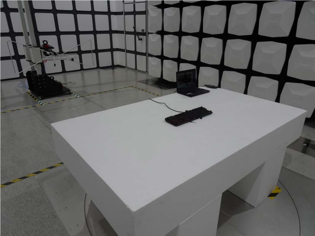
Front View of Radiated Test
