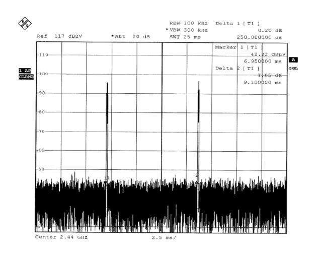
$20\log(\text{Duty cycle}) = 20\log\frac{0.25 \text{ ms}}{9.1 \text{ ms}} = -31.22\text{dB}$
