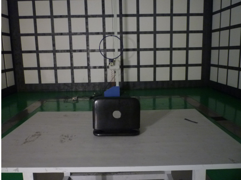
Photograph 2: Set-up for Spurious Emissions (30MHz-1GHz)
