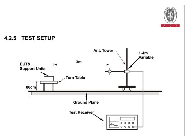
For the actual test configuration, please refer to the attached file (Test Setup Photo).
