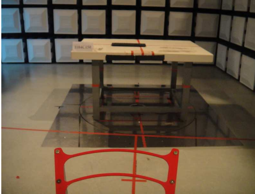
Photograph 3: Set-up for Radiated Emissions (1GHz-26GHz)
