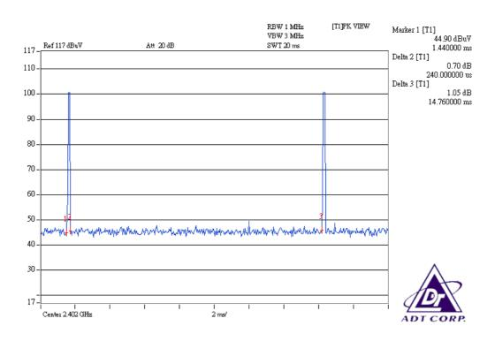
$$20\log(\text{Duty cycle}) = 20\log\frac{0.24 \text{ ms}}{14.76 \text{ ms}} = -35.78 \text{dB}$$
