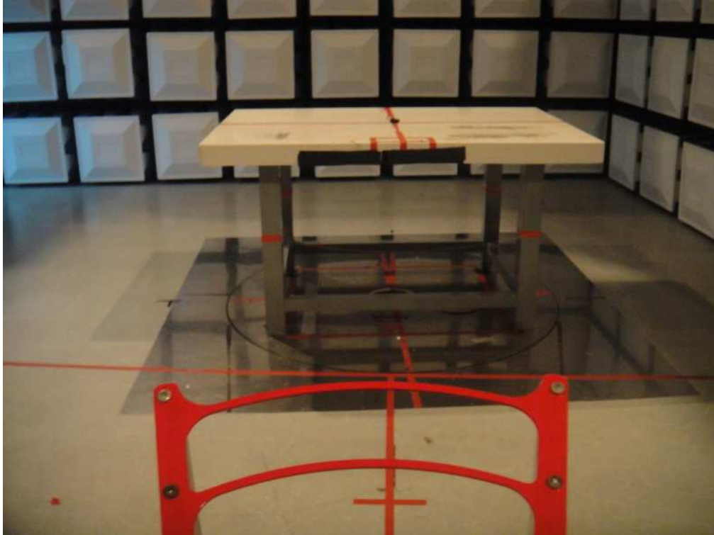
Photograph 5: Set-up for Spurious Emissions (1GHz-26GHz)
