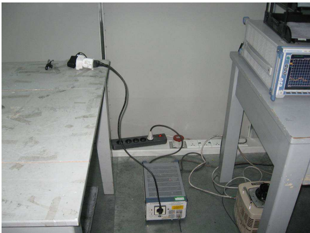
Photograph 2: Set-up for Conducted Emissions
