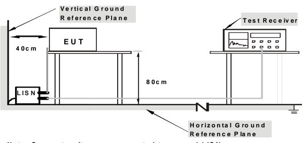
Note: Support units were connected to second LISN. For the actual test configuration, please refer to the related item – Photographs of the Test Configuration.
