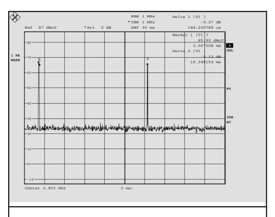
$20 \log (Duty cycle) = 20 \log (0.144 \text{ ms} / 16.346 \text{ ms}) = -41.1 \text{ dB}$
