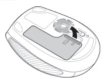
2 Pull the dongle out of the battery compartment.
