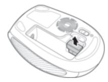
3 Insert one AA battery into the battery compartment. Make sure that the + and – symbols on the battery match the + and – symbols in the battery compartment.
