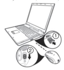
2 Slide the power button on the bottom of the mouse down to turn on the mouse. The laptop detects the mouse.
