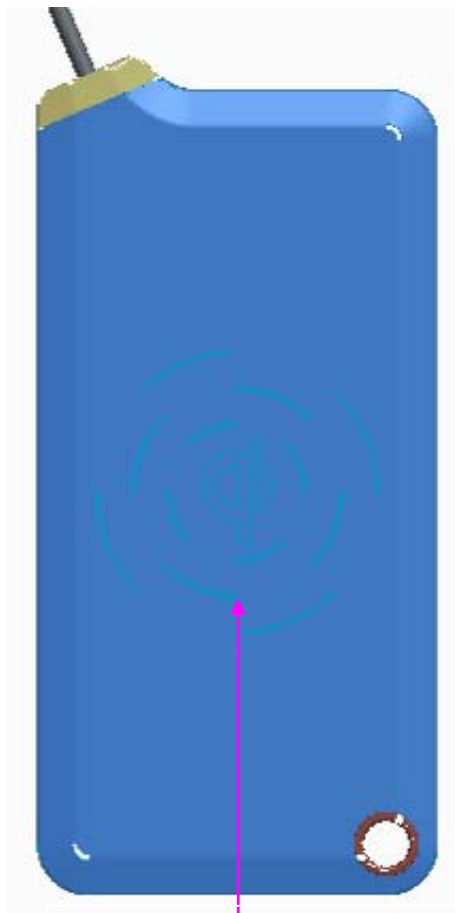
Charging Area and Transmitter Coil location of Wireless Charging Pad
