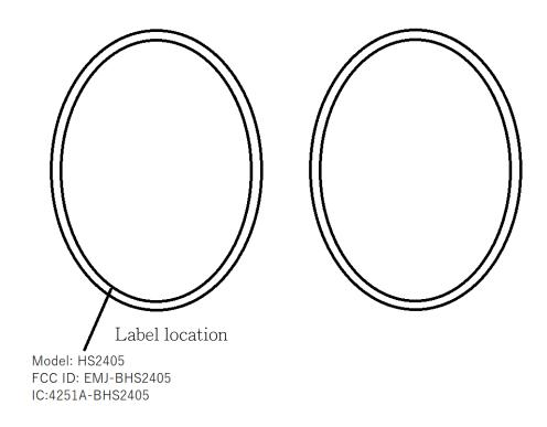
The label is permanently affixed on the interior of the earcup. The earcup cover can be opened without any special tools. Page 4 of the user manual exhibit provides instructions to the end-user on how to remove the earcups to view the regulatory label containing the FCC / ISED ID. The FCC / ISED ID will also be placed in the owner's guide.
