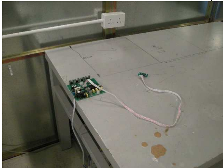
Measurement of Conducted Emission Test Set Up
