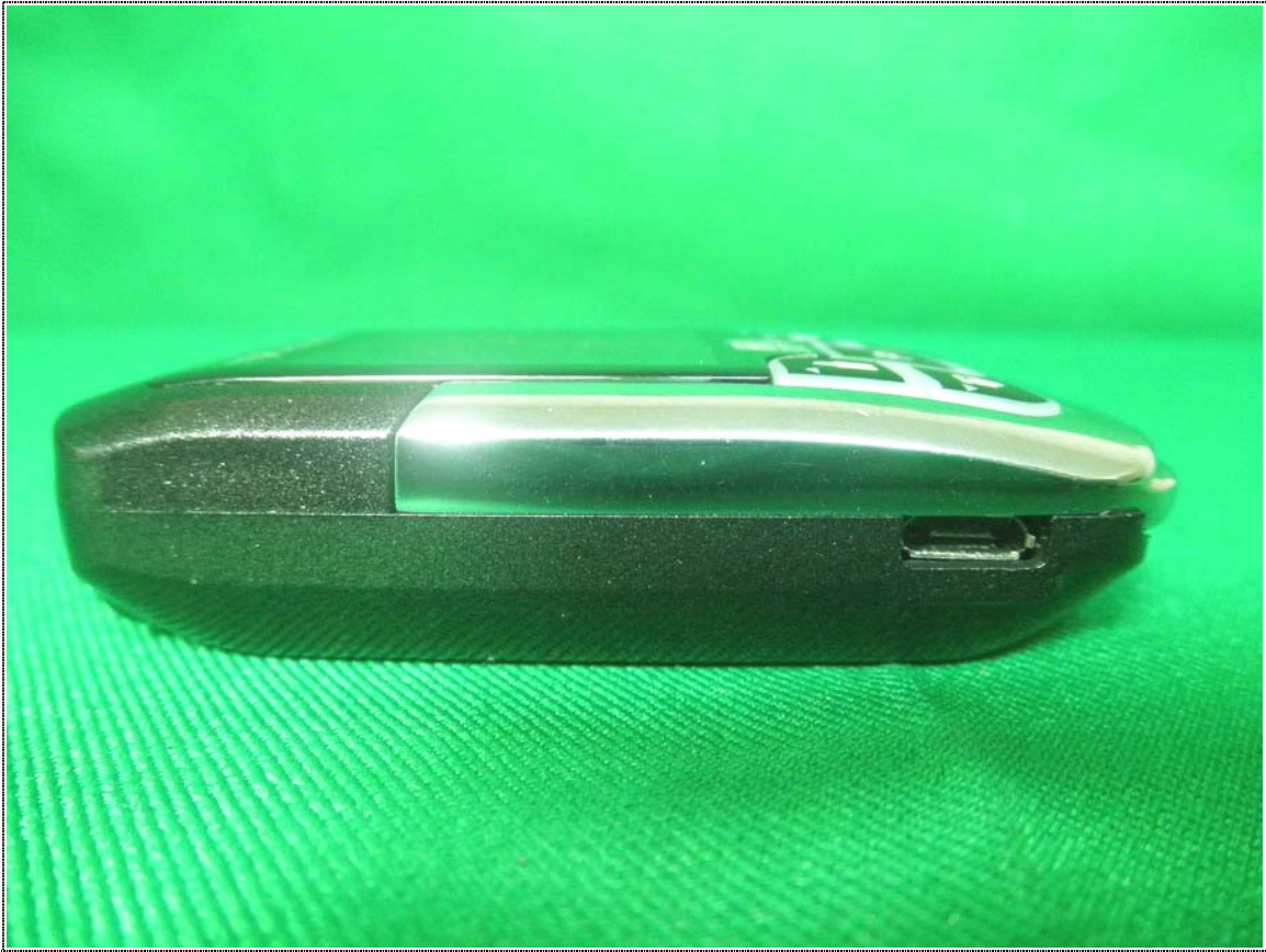
View of I/O Port
