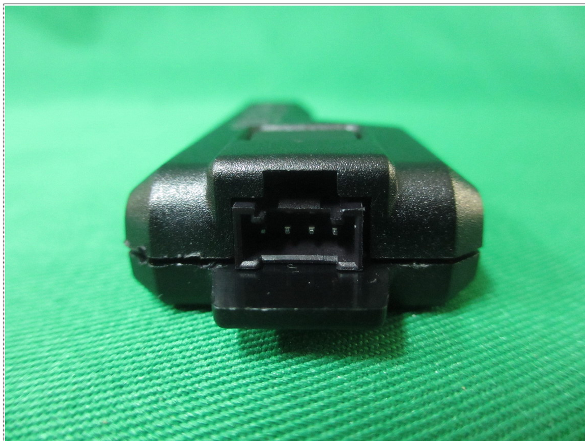
View of Power port
