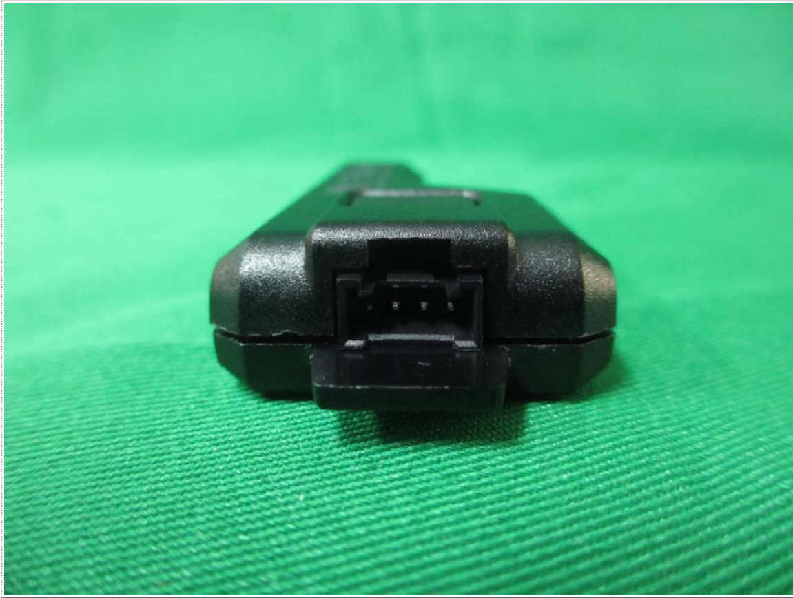
View of Power port
